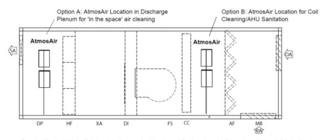
Example of Bipolar Ionization Tube installation in a generic air handling unit (for illustration only). Source: https://d3ciwvs59ifrt8.cloudfront. net/a02e5a7a-d7d4-4460-b933-6a0c761e7ef1/1d3eb8b6-9fda-498c-89fe-cd6e01c9dde2.pdf
